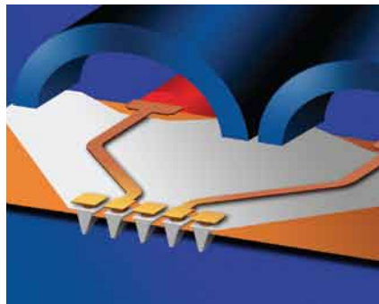
The microstrip extends all the way to the probe tips
